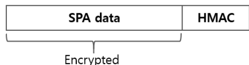
Fig. 3. Simplified SPA message structure
